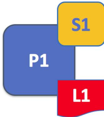
A peer hosts instances of ledgers and instances of chaincodes. In this example, P1 hosts an instance of ledger L1 and an instance of chaincode S1. *There can be many ledgers and chaincodes hosted on an individual peer.*
