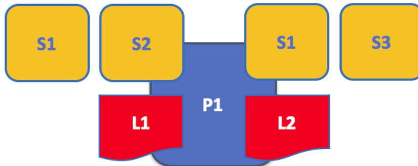
*An example of a peer hosting multiple chaincodes. Each ledger can have many chaincodes which access it. In this example, we can see that peer P1 hosts ledgers L1 and L2, where L1 is accessed by chaincodes S1 and S2, and L2 is accessed by S1 and S3. We can see that S1 can access both L1 and L2.*
