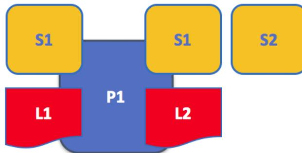
A peer hosting multiple ledgers. Peers host one or more ledgers, and each ledger has zero or more chaincodes that apply to them. In this example, we can see that the peer P1 hosts ledgers L1 and L2. Ledger L1 is accessed using chaincode S1. Ledger L2 on the other hand can be accessed using chaincodes S1 and S2.
