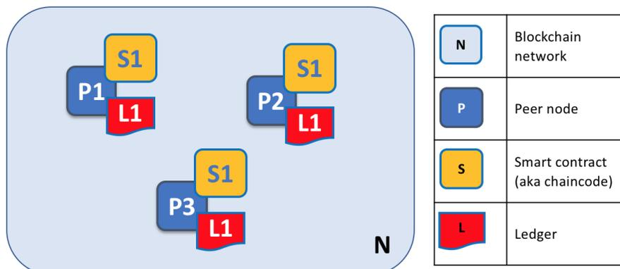
*A blockchain network is comprised of peer nodes, each of which can hold copies of ledgers and copies of smart contracts. In this example, the network N consists of peers P1, P2 and P3, each of which maintain their own instance of the distributed ledger L1. P1, P2 and P3 use the same chaincode, S1, to access their copy of that distributed ledger.*
